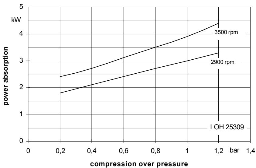
The values indicated for volume flow and power absorption are valid for compression of dry air at 20°C from atmospheric pressure (1013 mbar) to the respective compression pressure with water at 20°C as service liquid. Tolerance of the curve values is 10 %. The compression pressure in bar is indicated as pressure above the atmospheric pressure.
