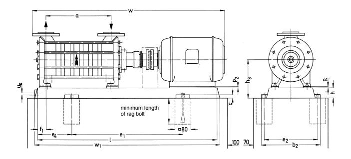
Dimensions in mm, dimensional tolerances admissible (base plate) for castings acc. DIN 1686 / GTB 16/5, for welded parts acc. DIN 8570 B.
