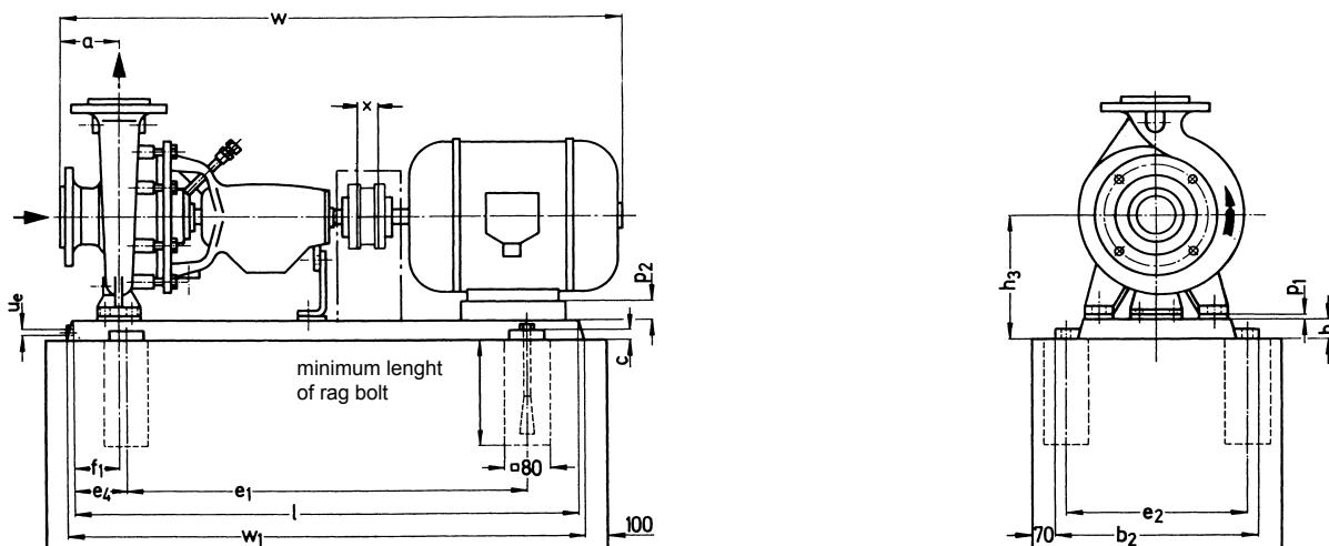
Dimensions in mm, tolerances (base plates) for cast pieces acc. to DIN 1686/GTB 17,
