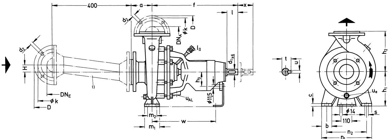
I<sub>II</sub> = connection for air ventilation pipe G 3/8
