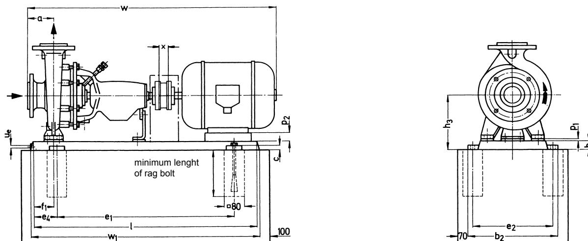
Dimensions in mm, tolerances (base plate) for cast pieces acc. to DIN 1686/GTB 17,
